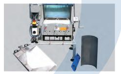
Due to the Quick snap fasteners used on the GSL series machines, the machines can be opened for cleaning and maintenance quickly without the need for special tools.
